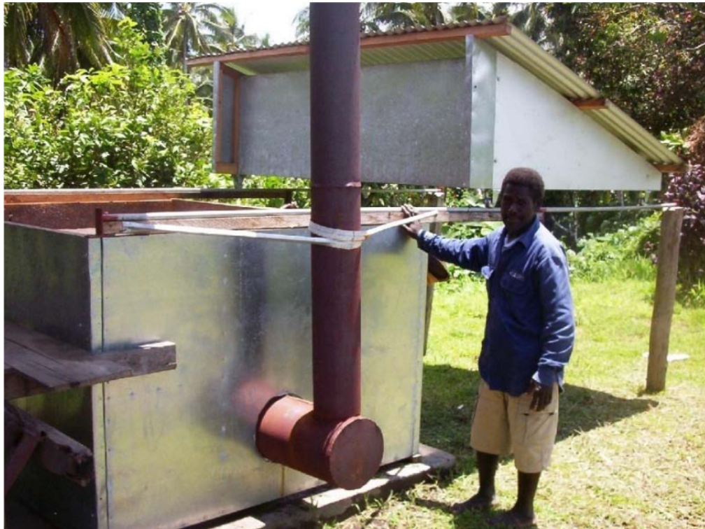
Plate 5-1 Mini-dryer used in Solomon Islands for cocoa drying
