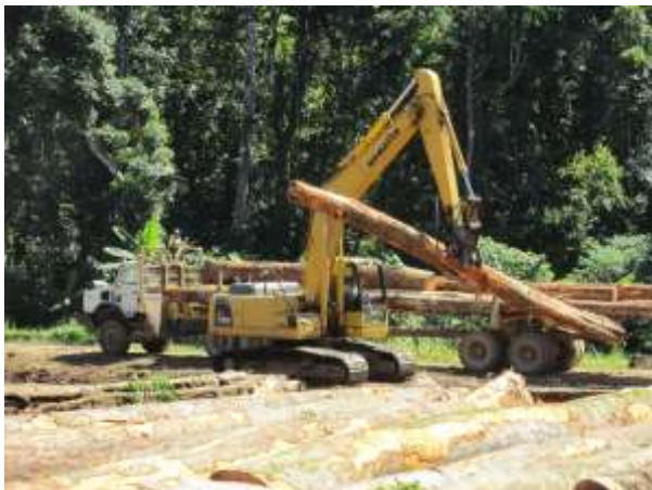
Figure 10: A log truck with a payload capacity of 25 to 30 m 3 of logs. 500 m 3 /y would equate to 17 to 20 such truckloads of logs processed per year.
