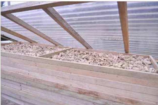
A cover made with a wooden frame and clear perspex being placed on a stack of drying racks to protect the racks from the rain
