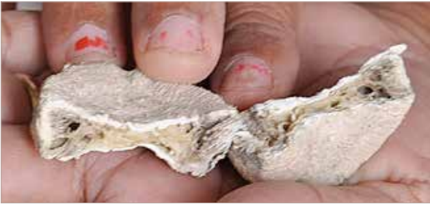
Badly dried material showing soft interior
