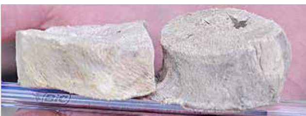
Dried material that has been rewashed and redried (left) and not rewashed (right)
