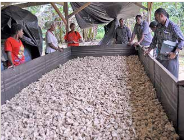
A diesel-powered drying chamber uncovered to show dried material
