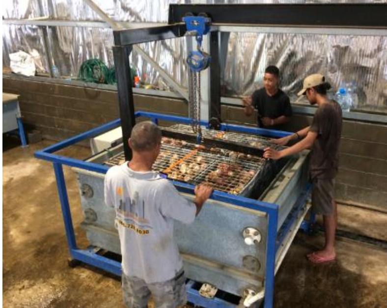
Figure 5. Pilot-scale hot water treatment (48°C) of approx. 200 kg of taro in 12 plastic crates. Water is pumped under the crates, flows up the stack and over the top where it flows over a weir and is heated using electric elements.
