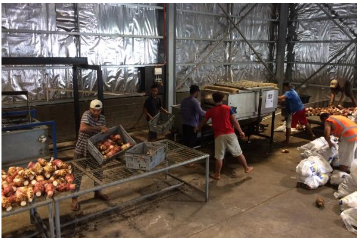
Figure 7. Overview of Ah Liki staff carrying out the treatment process. Incoming taro on the right (bagged and in the flume (top right), high pressure washer (middle- right), hot water bath (left), and taro drying on racks (bottom left).
