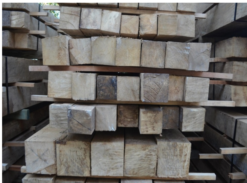
Plate 4-6 Imported Vitex flitches, racked and being air-dried, Queensland (note the variable dimensions and rough ends of the timber)
