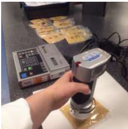
Figure 19. The experimental setup for measuring the colour of the ginger paste
