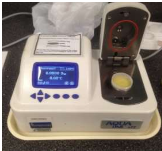
Figure 13. The experimental setup used to measure water activity
