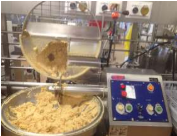
Figure 17. The bowl chopper showing the peeled ginger paste before acid and preservative addition
