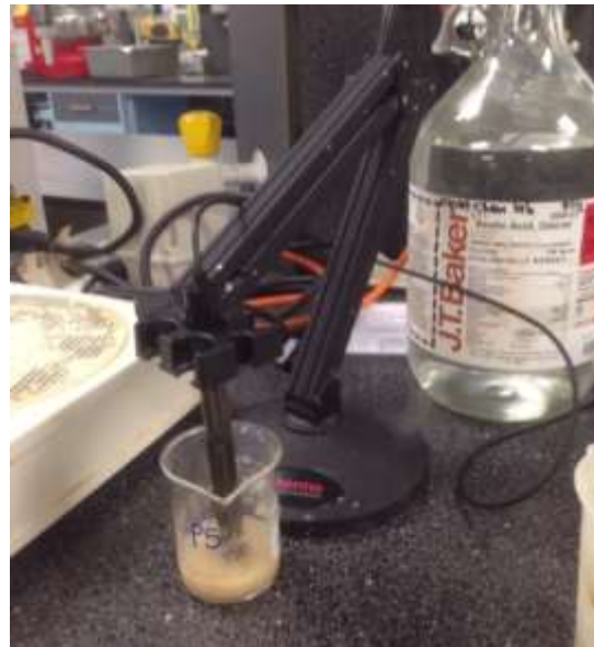
Figure 14. The experimental setup used for measuring pH
