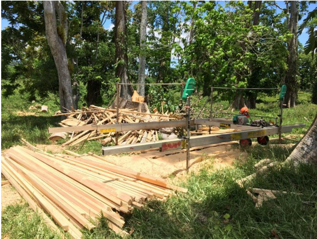
Figure 2-1 Typical portable mill set up on Efate, processing melek trees on farms
