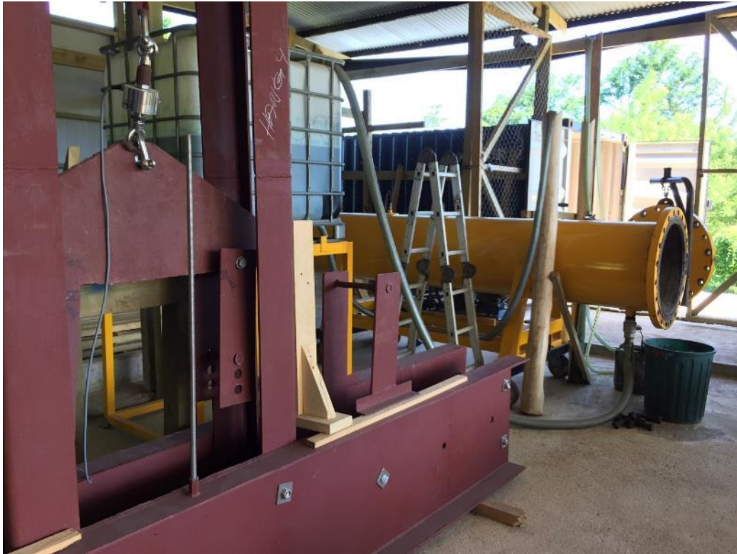
Figure 3-2 Timber Research Facility on Santo set up with portable pressure treatment tank for treating Whitewood
