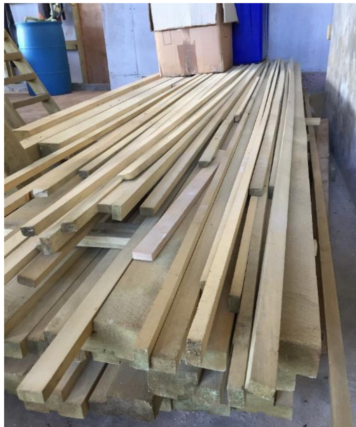
Figure 3-3 Vanuatu Whitewood sawn timber treated at the Timber Research Facility on Santo
