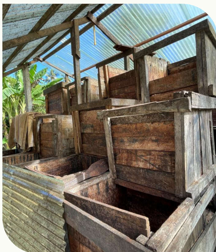
Photo: Cascading cocoa bean fermentation boxes developed with and for a farmer with physical disabilities to enable him to perform his duties efficiently and effectively. Source: Gaston Chocolat.
