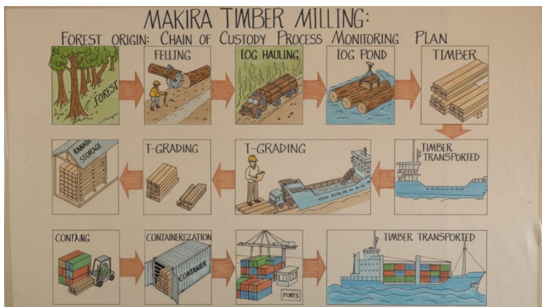
Figure 3: Sawn timber value chain, hanging on the walls of Align Timber Milling
